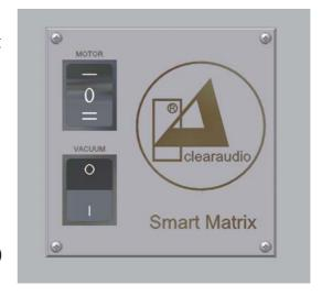
Using the "VACUUM" switch the vacuum process will be started.
